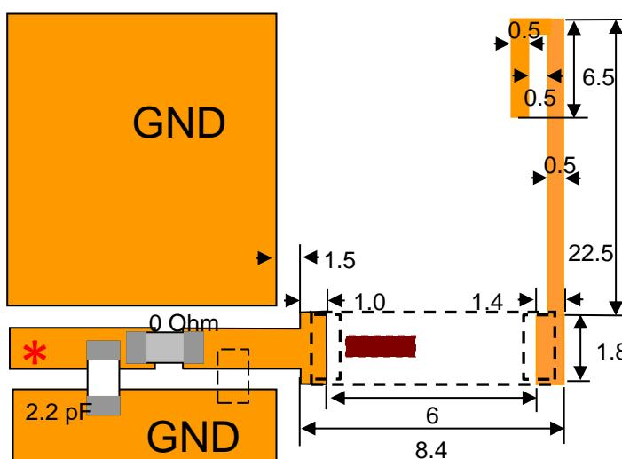
\* Line width should be designed to match 50ohm characteristic impedance, depending on your PCB material and thickness (distance to GND)
