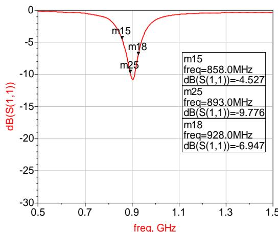
This antenna has about 20MHz of guard-band on each side
