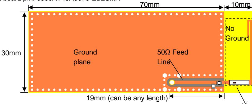
• Orderable EVB for evaluation, it comes with a female SMA connector. Go to: [www.johansontechnology.com/request-a-sample](http://www.johansontechnology.com/request-a-sample) and ask for p/n 0900AT43A0070-EB2SMA
