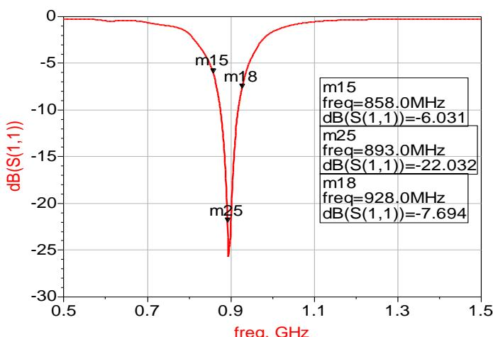
This antenna has about 20MHz of guard-band on each side
