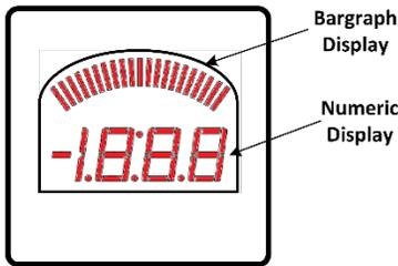
**Bar-graph Display:** The 21 segment bar-graph display responds quickly and smoothly like an analog meter movement to aid in reading rapidly changing measurements.
