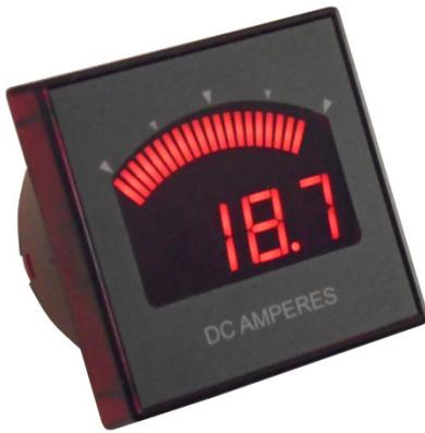
The DMR35-DCA series of panel meter performs precision measurements of DC current and is available in two models offering ranges from 1A to 25A. The 3-1/2 digit numeric display supports precision measurement, and a fast-responding 21 segment bargraph tracks quickly-changing measured values.
