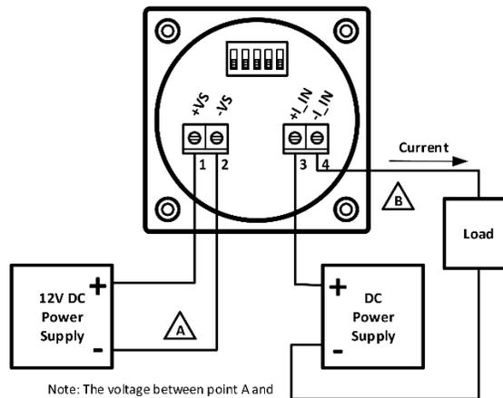
Note: The voltage between point A and point B must be within  $\pm 48V$
