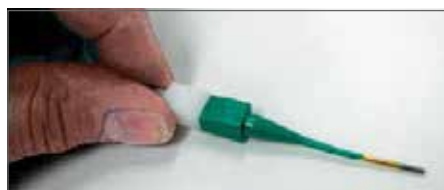
Plastic tool with contact in proper position.
