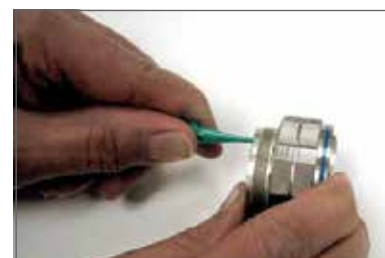
Plastic tool with contact in proper position.
